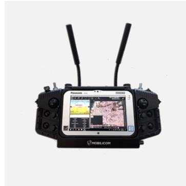
Ground Control Stations
